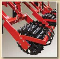
Individual spring loaded heavy cast Prisma press rollers follow immediately behind each leg to close and level the surface leaving your field ready for use.
