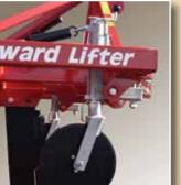
Spring loaded cutting discs in front of each leg on galvanized manual winding depth adjusters cut through the grass sward preventing damage and soil bursting to the
