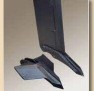
The front of the leg has a replaceable, reversible shin to keep the cost of metal wear as low as possible. Two cast point options consist of the 6cm standard and a 25cm winged point to suit all conditions and soil types.
