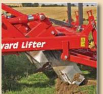
Leg protection is provided by either shearbolts or a hydraulic auto-reset system to prevent damage from large obstacles under ground.
